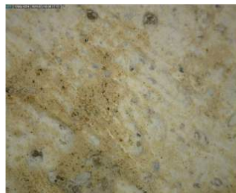
Fig.62. Detail of type two stucco (Dino-Lite image, 50x inc)
