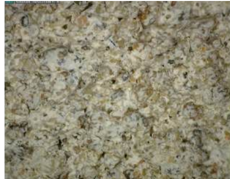
Fig.60. Detail of the mortar used for the grouting of the apse (Dino-Lite image, 50xinc).
