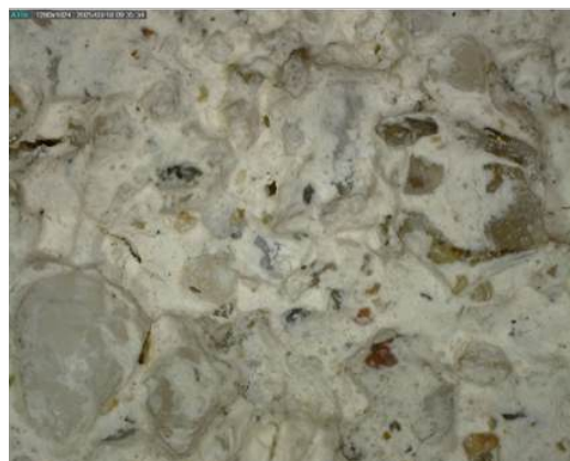
Fig. 57. Details of the filling (Dino-Lite image, 50x zoom inc)
