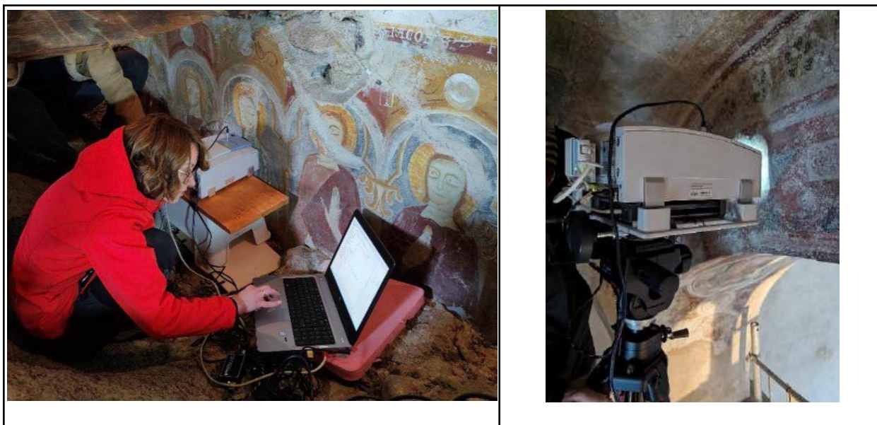
Figure 1 – Images of the portable FT-IR spectrophotometer ALPHA II (Bruker Optics): setup and distance of the instrument from the investigated surface.
