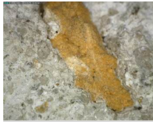
Fig.36. Dino Lite (x50mag) picture of the additive (wood)
